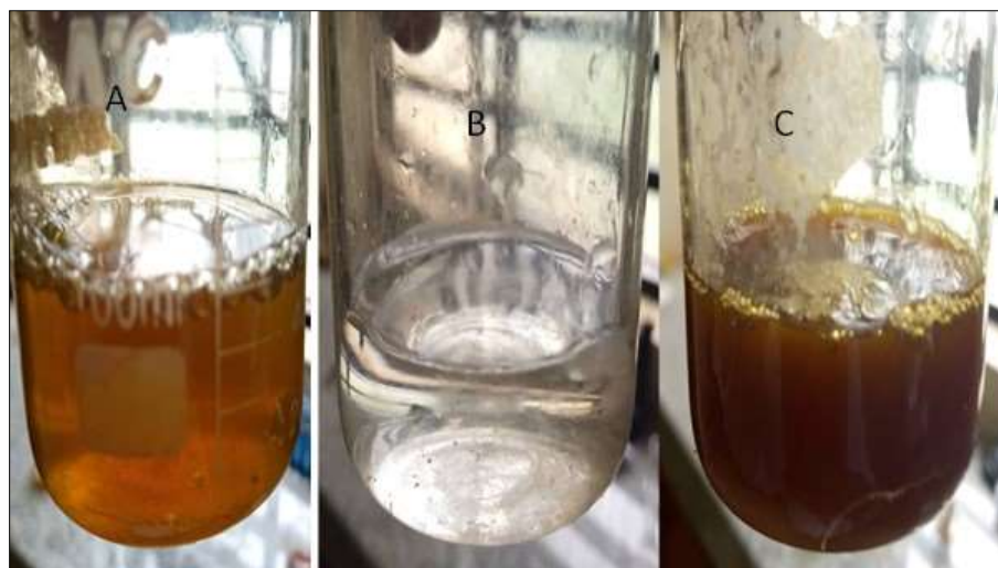
Fig 1: Color change of the reaction (A) plant extract (B) aluminum nitrate and (C) mixture containing nanoparticle
