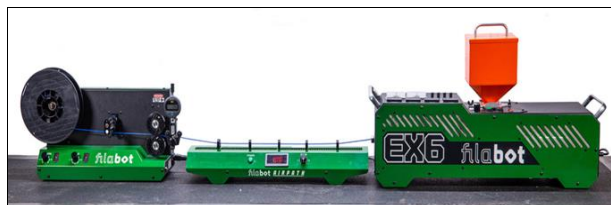
Fig 1: Extruder for the production of polymer threads
