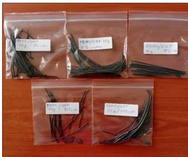
Fig 4: Filaments of graphene/polymer composites made by extruder
