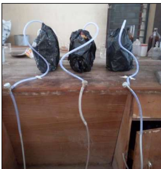
Fig 3: Digesters on Stand During Digestion Process
